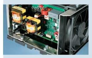
**Compact.** High-frequency transformer technology makes these devices remarkably light, compact and simple to install.
