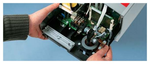
**On-site service.** The modular design of the inverter and on-site servicing by our engineers will keep your system up and running. Circuit board replaced – the inverter is working perfectly again immediately.
